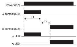
%T 1: Setting time (\$\( \Lambda \) contact operation time ) %T2: \$\( \Lambda - \Delta \) Swtiching time (\$\( \Lambda \) and \$\( \Delta \) contact are OFF when power is ON.)
