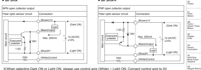
When selecting Dark ON or Light ON, please use control wire (White) Light ON: Connect control wire to 0V Dark ON: Connect control wire to +V
