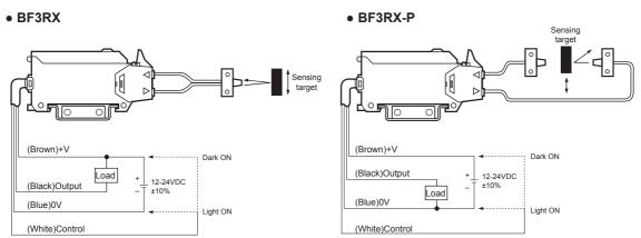
\*Enables to use diffuse reflective type or through-beam type according to the fiber optic cable.
