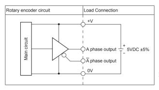
XAll output circuits of A,  $\overline{A}$ , B,  $\overline{B}$ , Z,  $\overline{Z}$  phase are same.
