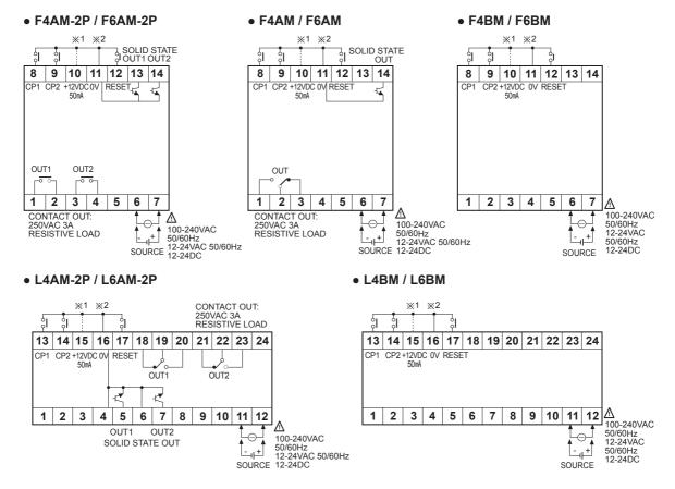
%1: Connection for PNP input in contact input
