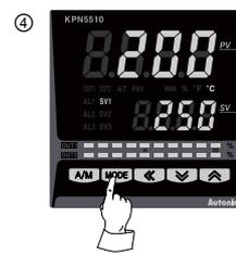
Press the **MODE** key to save the setting value. If there is no additional key operations in 3 sec., the changed SV is automatically saved.
