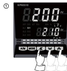
Press any key among the , , in RUN mode to enter into SV setting mode. Last digit (10<sup>0</sup> digit) on SV display part flashes.
