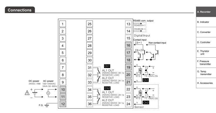
X Shaded terminals are for the standard model. (power terminal, CH1 input terminal, DI input terminal)
