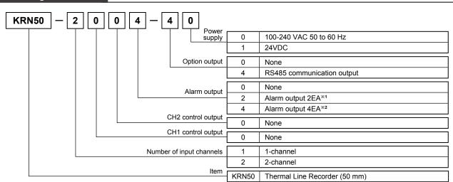
※ 1. When selecting this for 2 CH model, 2EA alarm outputs for CH1 are available. In other words, you cannot set 1EA for CH1 and 1EA for CH2.
