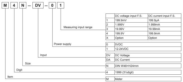
%M4N series is to measure DC only. AC voltage and AC current is not available to be measured. %Measuring range for direct connection is max. 200VDC, max. DC200mA.
