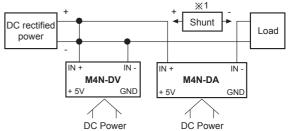
%1: If measure higher current than measuring input range, please use a shunt. If measure higher voltage than measuring input range, please use multiplier.
