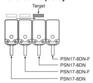
When installing several proximity sensor closely, it may cause malfunction due to mutual interference. Therefore, please use differential frequency for the application XDifferential frequency type is only for 17 square.
