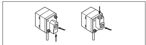
3. Please use seal tape at port plug in order to prevent pressure leak.
