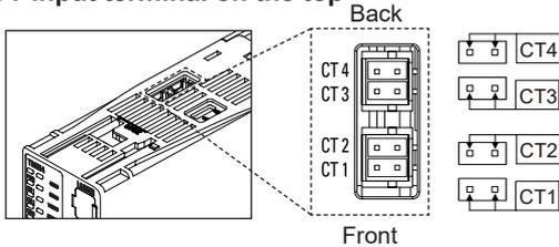
※ When use the CT input terminals, remove the robber cap.
